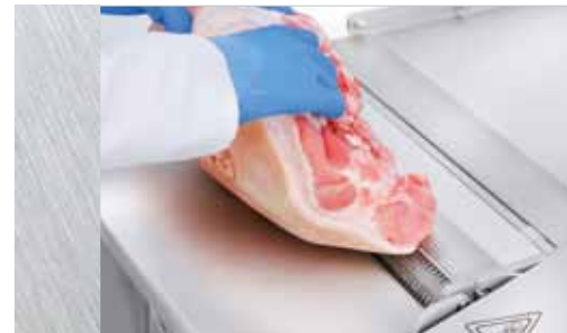
ESM 5550: Manual derinding of round cuts (standard infeed table "straight")
